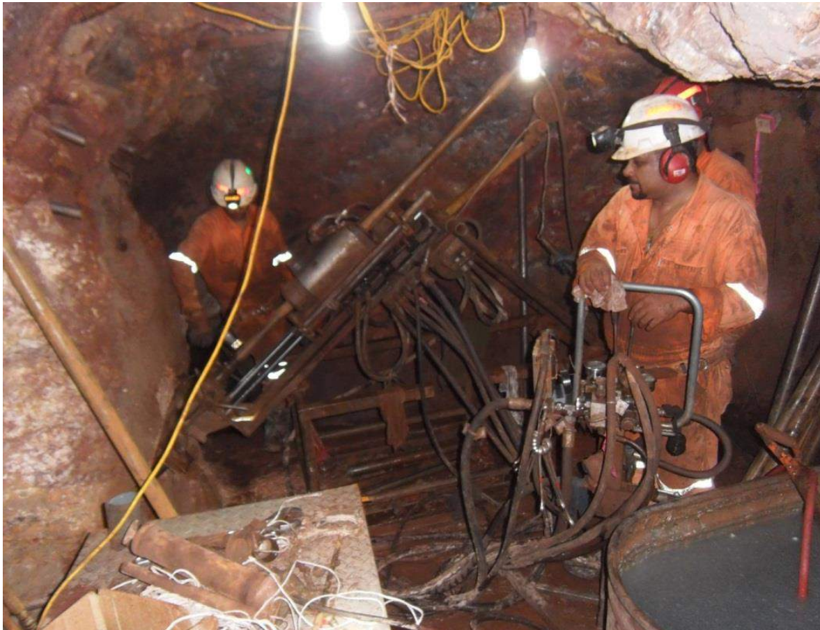
Figure 10-2. Typical Set-Up of the Termite Drill during the Long Hole Twin Program, 2012-2013
